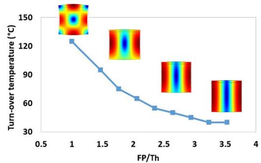
Fig. 3. The simulated turnover temperature of a QTL TPOs resonator as a function of finger pitch to stack thickness ratio [5].
