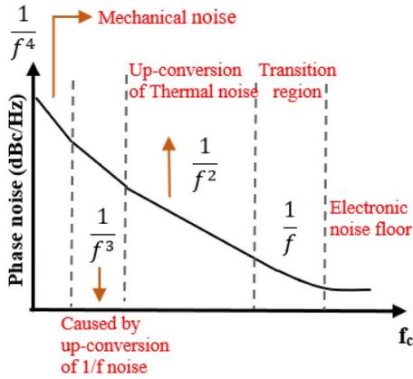
Fig. 1. The phase-noise spectrum of a typical feedback oscillator.
