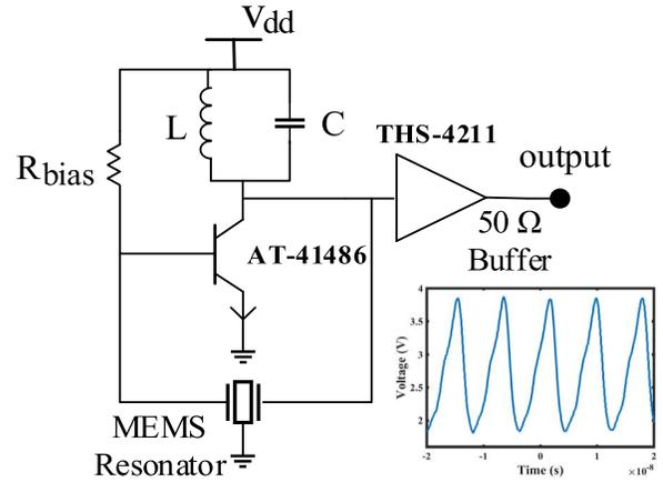
Fig. 6. Schematic of the oscillator circuit and the measured output waveform.
