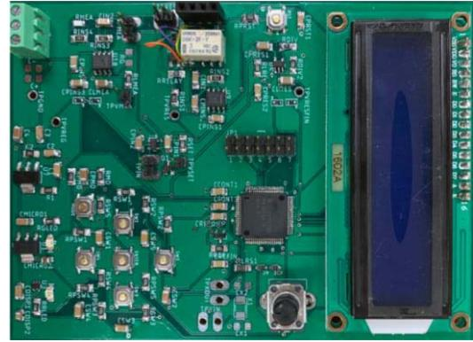
Fig. 9. The printed circuit board of a custom-made micro-controlled based temperature controlling circuit.
