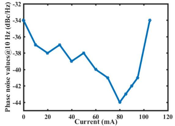
Fig. 12. Measured phase noise @10Hz carrier offset for different amount of current injected in the resonator.
