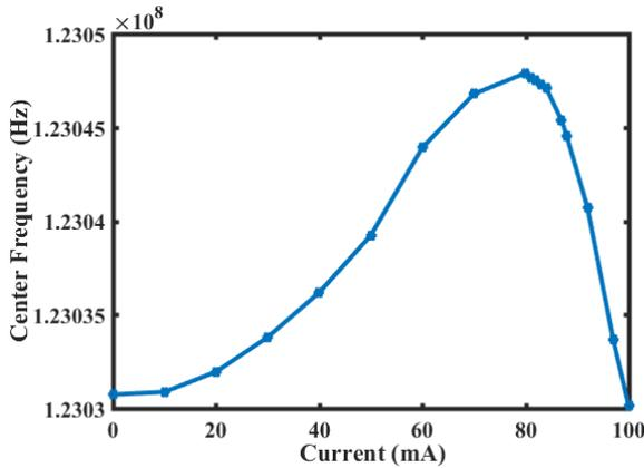
Fig. 10. The variation of center frequency versus the current injected through the silicon body of the resonator.
