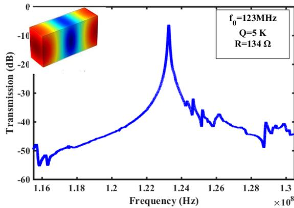
Fig. 5. Frequency response of the QTL-TPoS resonator and the stress-profile of the mode-shape.
