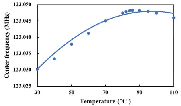
Fig. 7. The frequency vs. temperature plot exhibiting a turnover temperature at  $\sim 90^\circ\text{C}$ .
