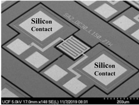
Fig. 4. The scanning electron micrograph of the QTL-TPoS resonator with isolated contact to silicon body for injecting current to heat up the resonator.
