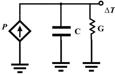
Fig. 8. Equivalent electrical circuit for the thermal diffusion of an resonator.
