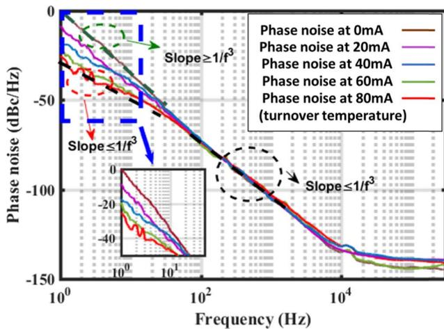
Fig. 11. The measured phase noise at different levels of injected current through the resonator.
