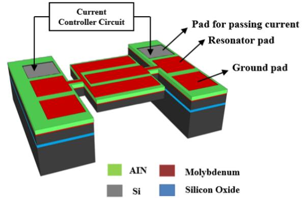
Fig. 2. The schematic of the quasi thickness-Lamé TPOs (QTL-TPOs) resonator highlighting the pads for injection of a DC current through silicon body to efficiently heat the resonator.
